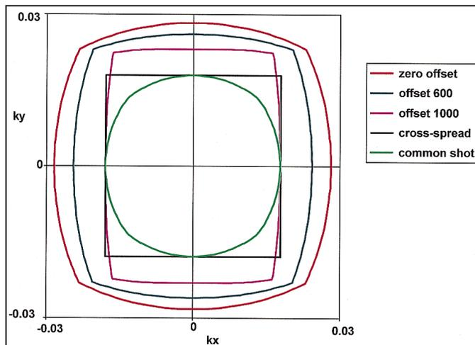
**Fold.** The migration formulas do not cater for overlapping single-fold data sets. As a consequence, the potential resolution of multi-fold data is some average of the potential resolutions of the contributing single-fold data (see below). Yet, fold improves achievable resolution.
