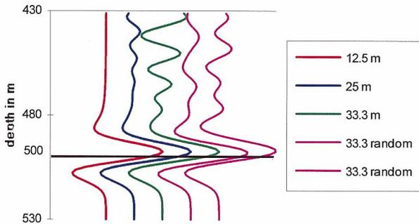
**Bin fractionation.** On the right (top), conventional sampling is compared with sampling using the bin-fractionation technique. The station spacings in the two sampling techniques are the same, but in the bin-fractionation technique the midpoint spacing is smaller. The question is, does this lead to better resolution?
