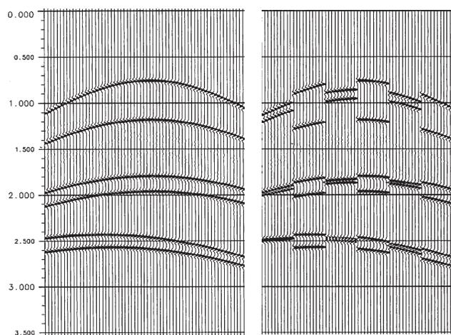
**Figure 4. Continuous shot lines (left) vs. bricked shot lines (right), showing that the latter produce edges and reduce spatial continuity. Vertical axis is in seconds.**
