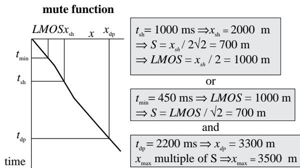
Figure 9. Example of determination of line interval
