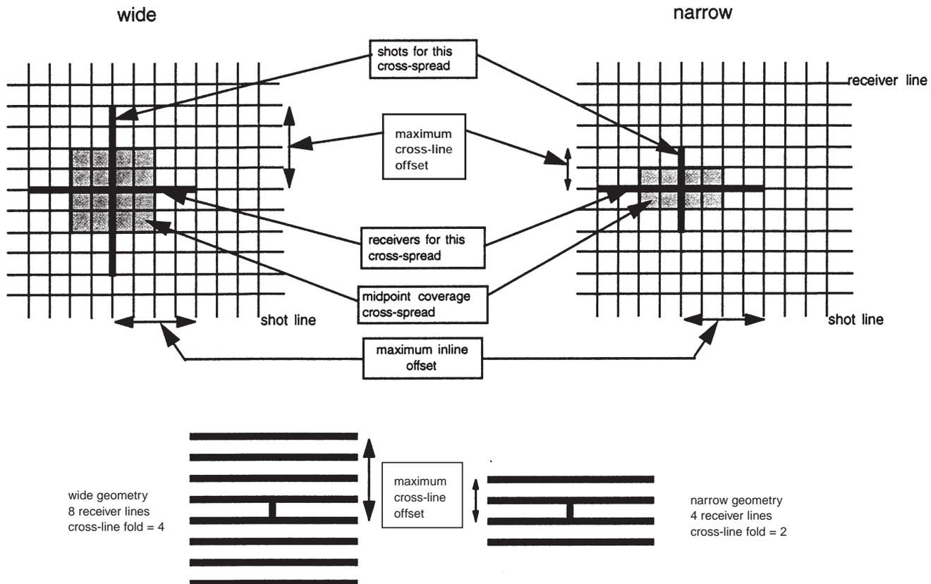
Figure 1. Narrow vs. wide geometries. Acquisition lines with cross-spreads (top) and corresponding generating swaths (bottom).
