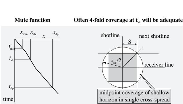
Figure 7. Determination of line interval and maximum offset.
