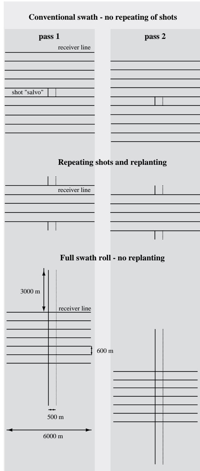
Figure 12. Same nominal geometry can be realized with different swath arrangements.
