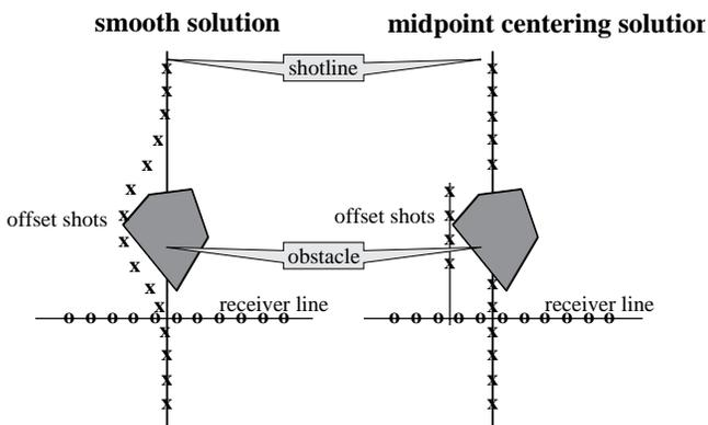
Figure 10. Avoiding data gaps due to obstructions.
