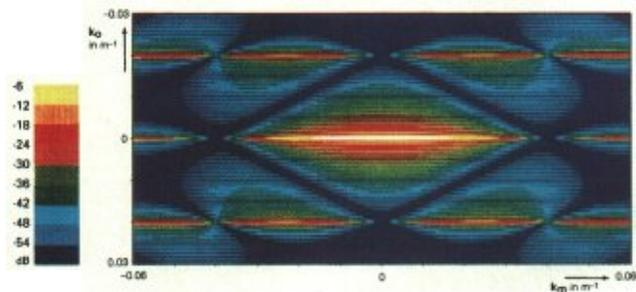
Figure 14. Total stack response for a symmetric sampling technique. The notches of the CMP array run parallel to the  $k_m$  axis.
