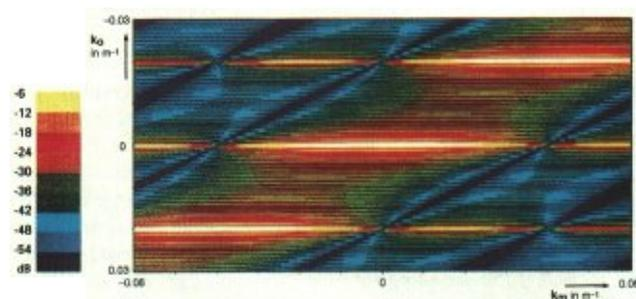
Figure 15. Total stack response for an asymmetric sampling technique without a shot array. Note the greatly reduced suppression and the asymmetry in the response.
