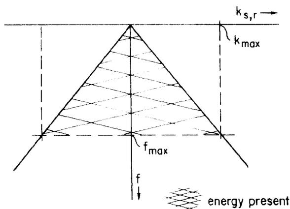
**Figure 7.** Regions with and without energy in  $f, k_s$  and  $f, k_r$ . Maximum frequency of event with minimum phase velocity determines maximum wavenumber and it is the same for shot and receiver coordinate.
