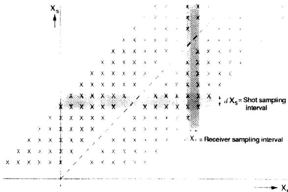
**Figure 5.** Shot and receiver sampling intervals in the surface diagram.
