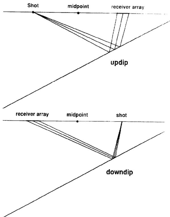
**Figure 10.** Updip versus down-dip shooting for an asymmetric configuration with a geophone array but no shot array.
