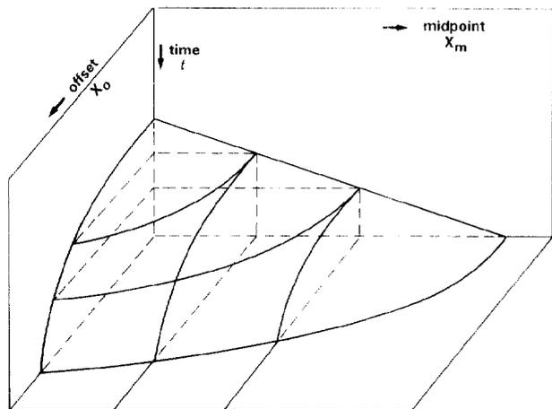
**Figure 3. Dipping event in midpoint/offset coordinate systems. The event is a hyperbola in the common offset panels (a straight line for zero offset), a hyperbola in the CMP, and an ellipse in the time slice.**
