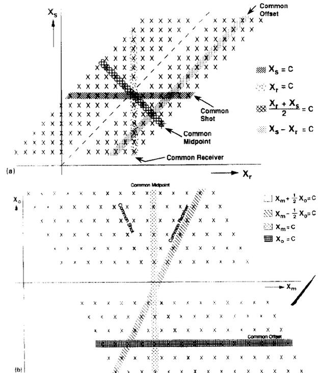
Figure 2. Descriptions of prestack seismic data set in (a) shot/receiver coordinate systems and (b) midpoint/offset coordinate systems. The former is also called a surface diagram and the latter a subsurface diagram or stacking diagram.
