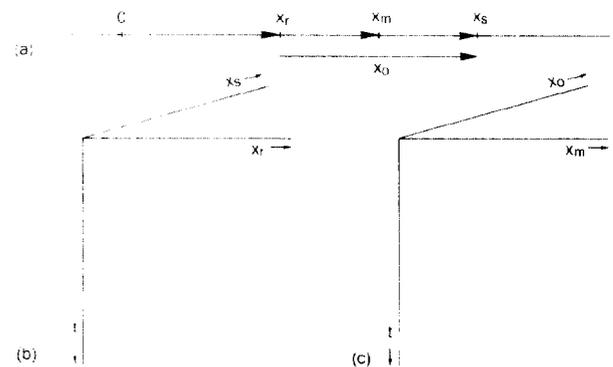
Figure 1. Prestack data coordinate systems. (a) The four spatial coordinates in relation to the seismic line. (b) Shot/receiver coordinate system. (c) Midpoint/offset coordinate system.
