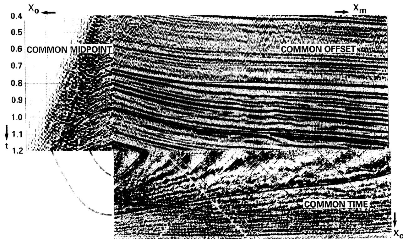
**Figure 4. Three cross sections through real prestack data set. Note that each event is a surface in 3-D  $t, x_m, x_o$  space.**
