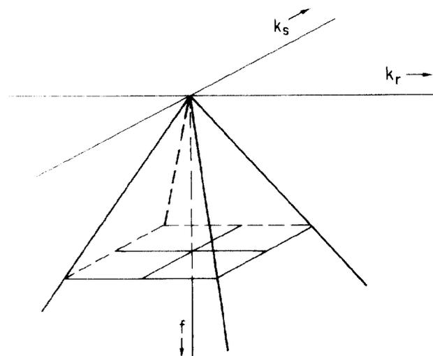
**Figure 8.** Energy of prestack data wavefield is confined to pyramid shaped volume in  $f, k_s, k_r$ . Base of pyramid is at  $f = f_{max}$ .
