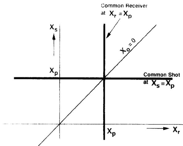
**Figure 6.** Common shot gather at  $x_r = x_p$  and common receiver gather at  $x_s = x_p$  are identical because of reciprocity.
