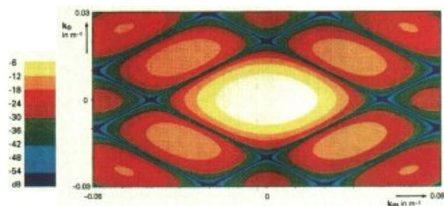
Figure 13. Combined response of shot and receiver arrays in midpoint/offset wavenumber domain. Oblique dark blue lines represent notches in the shot array and receiver array responses.
