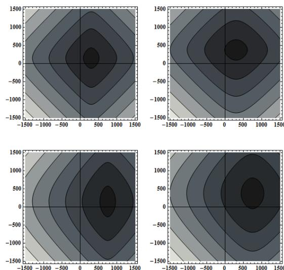
Fig. 1. Contour plots of traveltimes surfaces in midpoint domain of 4 surface scatterers in cross-spread. The scatterers are located at  $(x, y) = (600, 300)$  and  $(600, 750)$  in top row and at  $(1500, 300)$  and  $(1500, 750)$  in bottom row. First contour around apex of scatterer is at time of apex plus 250 ms, contour interval is 1000 ms.
