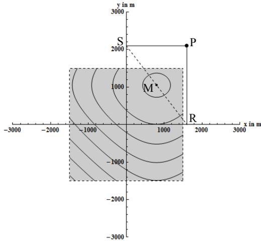
Fig. 2. Cross-spread used in Figure 1. A scatterer is located at (1600, 2100) and a contour plot of its corresponding traveltime surface is displayed in the gray midpoint area of the cross-spread. The travel path from shot S at (0, 2100) via scatterer at P to receiver R at (1600, 0) is the shortest path and the corresponding traveltime forms the apex of the traveltime surface.
