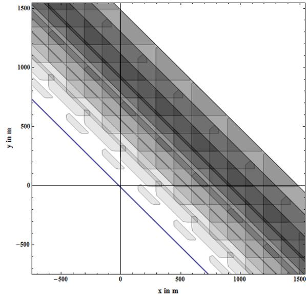
Fig. 5. Flattish apex areas of traveltimes contours for line scatterer (heavy line) in orthogonal geometry with 300-m line intervals. Cut-off velocity 2700 m/s, maximum time 3 s.
