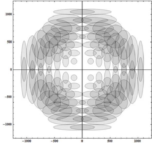
Fig. 3. Flat apex areas for single scatterer in origin in orthogonal geometry with 300-m line intervals.  $V_{\min,N} = 900$  m/s, cut-off velocity 2700 m/s, maximum time 3 s.
