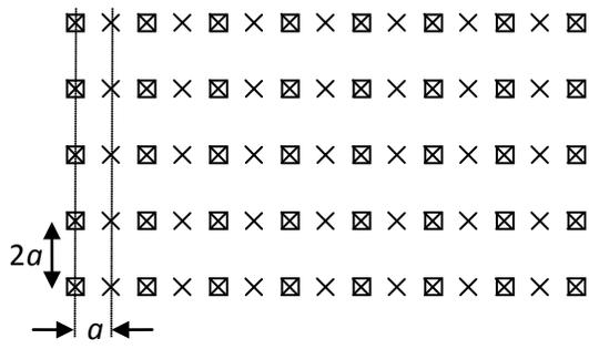
Figure 1. One implementation of Megabin. This geometry consists of a square ( $2a \times 2a$ ) grid of shots (squares) on top of a rectangular ( $a \times 2a$ ) grid of receivers (crosses).
