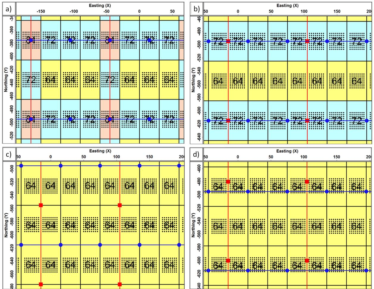
Figure 2. Offset-vector distributions in bins of various Megabin implementations. Red lines are shot lines, blue lines are receiver lines; red squares are shot locations, blue circles are receiver locations. Big black numbers indicate fold in bin. a) Standard Megabin implementation, all shots coincide with a receiver, b) Shots halfway receivers on the same receiver line, c) Shots halfway receivers and halfway between receiver lines, d) Shots not on receiver line, but close.
