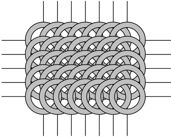
**Fig. 3. Offset range gather in orthogonal geometry. Each ring represents traces in midpoint domain with a narrow range of absolute offsets.**
