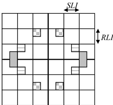
**Fig. 2. Cross-spread with some special case OVTs. Together, the two rectangular OVTs (dimension  $\frac{1}{2} SLI \times RLI$ ) can be used to construct an OVT gather with small spatial discontinuity between the OVTs. Together, the four chequered squares (dimension  $\frac{1}{2} SLI \times \frac{1}{2} RLI$ ) may be used to construct an OVT gather in case azimuth does not play a significant role. The eight small squares may be assigned the same mute time to achieve constant fold.**
