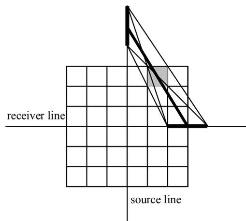
**Fig. 1. Offset-vector tile in cross-spread of 36-fold geometry. Heavy lines along source line and receiver line indicate range of shots and receivers contributing to OVT. Heavy line through middle of OVT indicates average offset and average shot/receiver azimuth.**
