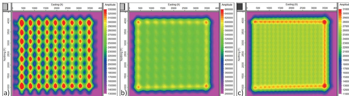
**Figure 2** Imaging of a reflector with  $15^\circ$  dip by OVT gathers in areal geometry. a) Horizon slice for  $400 \times 400$  m OVTs from upper right corner of 3D shot, b)  $400 \times 400$  m reciprocal OVTs from upper right and lower left combined, c)  $200 \times 200$  m OVTs from upper right corner of 3D shot.
