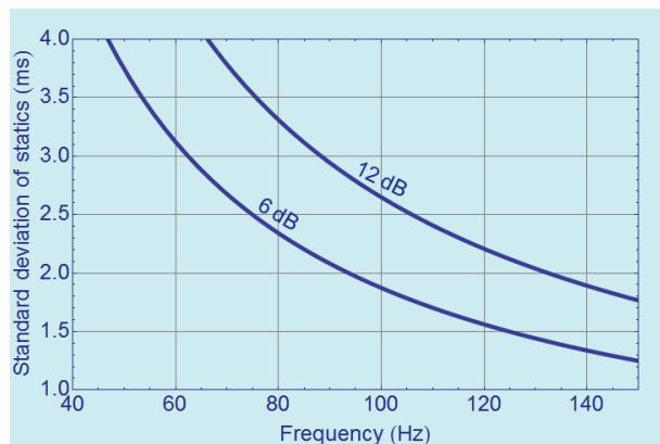
**Figure 1** Standard deviation in intra-array statics leading to 6 or 12 dB suppression as a function of frequency.
