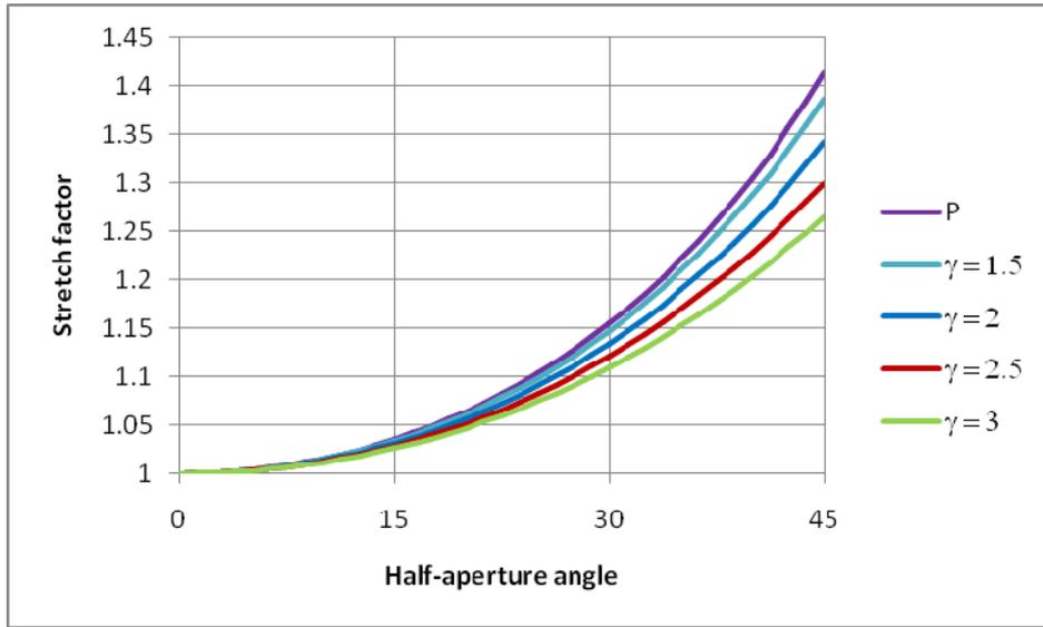
Fig. 5. NMO stretch factor as a function of half-aperture angle for various choices of  $\gamma$ . The curve labeled "P" is the same as in Figure 3.
