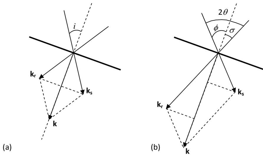
Fig. 1. Illustration of derivation of NMO stretch factor. (a) for P-waves, (b) for converted waves.
