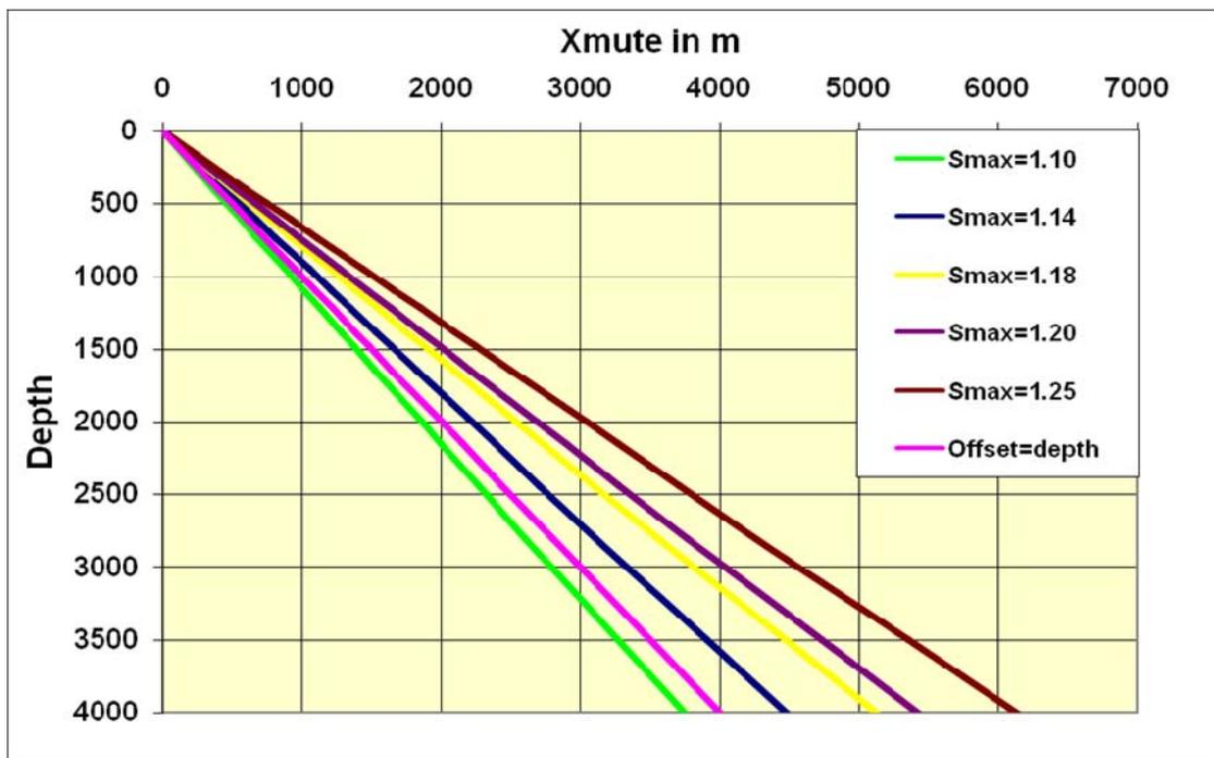
Fig. 4. Mute offset as function of depth for various maximum stretch factors.
