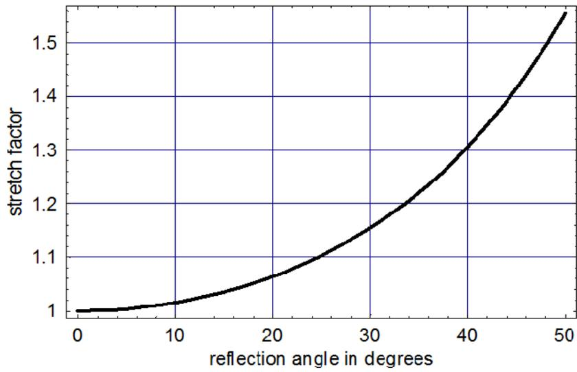
Fig. 3. Stretch factor as function of reflection angle.
