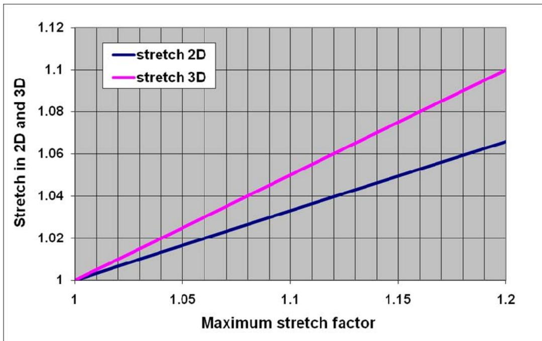
Fig. 2. Average stretch factors for 2D data and wide-azimuth 3D data as a function of the maximum stretch factor.
