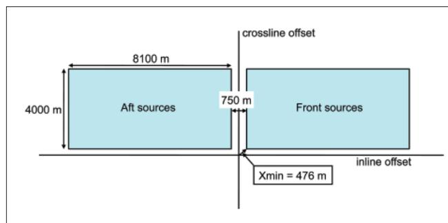
**Figure 2.** Offset and azimuth distribution of BP WATS configuration. Only positive crossline offsets larger than about 296 m are acquired. There is a 750-m gap in the middle of the range of inline offsets. Minimum absolute offset equals 476 m.
