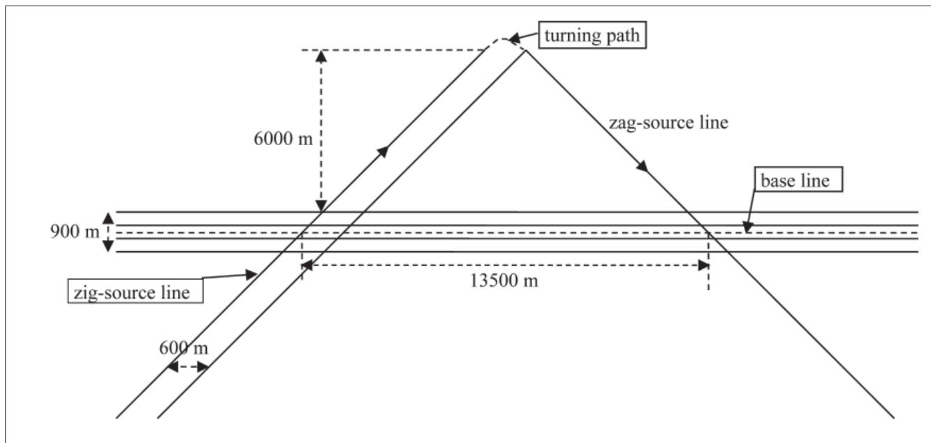
**Figure 7.** Wide-azimuth zig-zag geometry; 4 streamers @ 300 m. Maximum crossline offset 6000 m. Streamers to be towed deep enough to allow crossing with source vessel and sources (figure is not to scale). The source vessel is given 600 m in the inline direction to turn over 90° at the end of each shot line.
