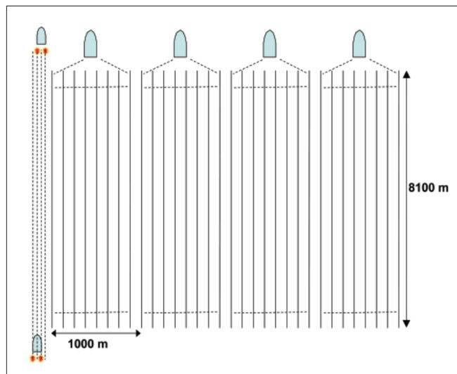
**Figure 1.** BP WATS configuration with two source vessels with two sources each and a single streamer vessel. The source vessels traverse the same source tracks four times while the streamer vessel moves up over 1000 m each time. Next the whole configuration moves up over 250 m in the crossline direction.
