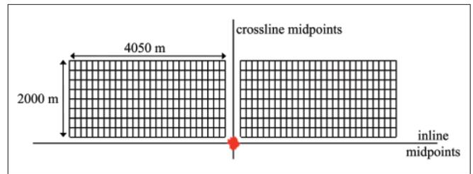
**Figure 3.** Quad-source midpoint area with OVTs in BP WATS configuration. Width of tiles in inline direction is  $4050/27 = 150$  m; in the crossline direction, the width is  $2000/8 = 250$  m.
