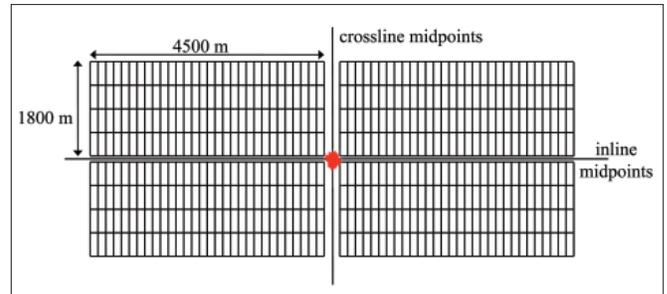
**Figure 4.** Quad-source midpoint area with OVTs in Shell WATS configuration. Width of tiles in inline direction is  $4500/30 = 150$  m; in the crossline direction, the width is  $1800/4 = 450$  m.
