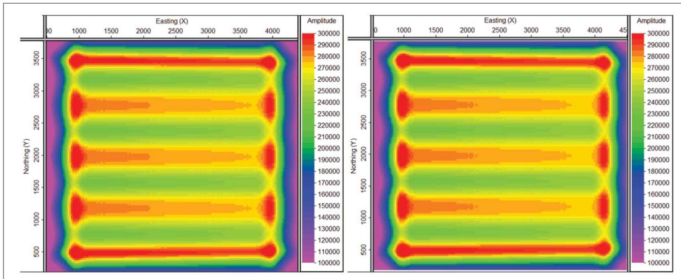
**Figure 5.** Horizon slices of migrated single-fold gathers for dipping event acquired with two different narrow-azimuth configurations. Left = 2 sources/8 streamers, right = 1 source/16 streamers. In both cases, nine antiparallel boat passes were acquired. The amplitudes in these two displays are virtually the same.
