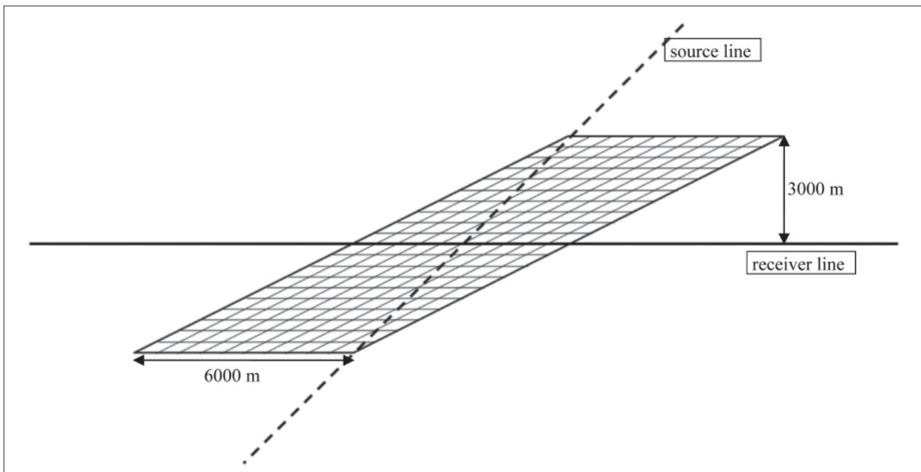
**Figure 8.** Zig-spread with offset-vector tiles for geometry with active spread length 12,000 m, maximum inline and crossline offset 6000 m, receiver-line interval 300 m, and source-line interval 600 m. There are 10 \* 20 OVTs in this zig-spread, corresponding to a fold of the zig-spreads only of 200. Adding zag-spreads would bring fold to 400.
