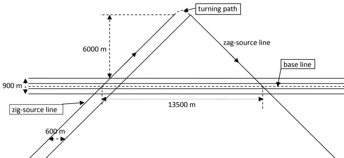
Figure 7. Wide-azimuth zigzag geometry. 4 streamers @ 300 m. Maximum crossline offset 6000 m. Streamers to be towed deep enough to allow crossing with source vessel and sources (Figure is not to scale). The source vessel is given 600 m in the inline direction to turn over  $90^\circ$  at the end of each shot line.
