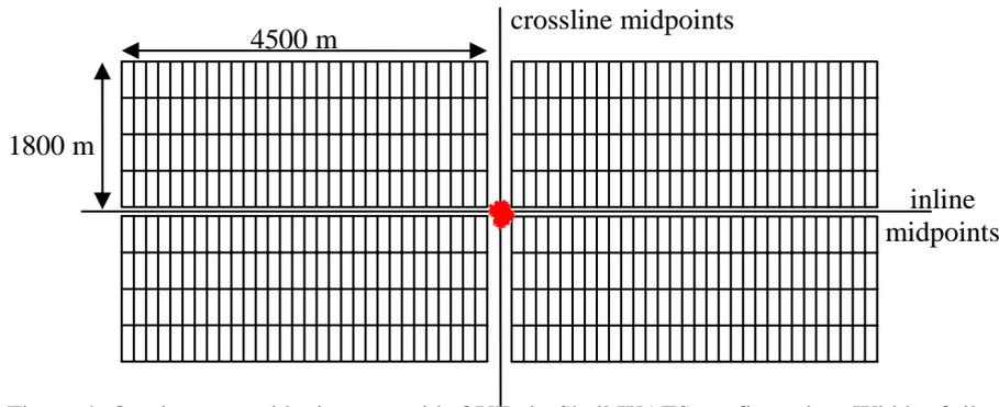
Figure 4. Quad-source midpoint area with OVTs in Shell WATS configuration. Width of tiles in inline direction is  $4500/30 = 150$  m; in the crossline direction the width is  $1800/4 = 450$  m.
