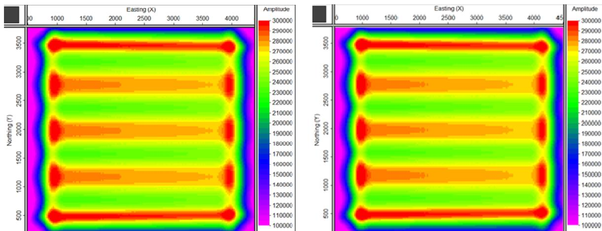
Figure 5. Horizon slices of migrated single-fold gathers for dipping event acquired with two different narrow-azimuth antiparallel configurations. Left: 2 sources / 8 streamers, right: one source / 16 streamers. The amplitudes in these two displays are virtually the same. The acquisition footprint is caused by the width of one boat pass (400 m in midpoints).
