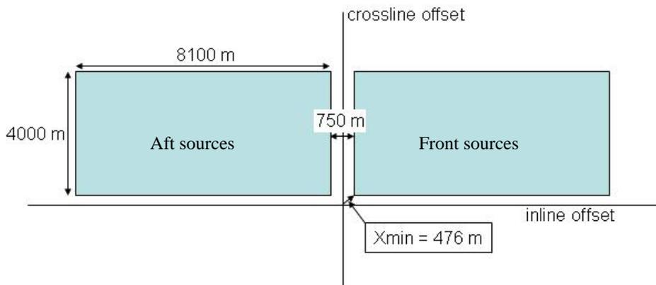
Figure 2. Offset and azimuth distribution of BP WATS configuration. Only positive crossline offsets larger than about 296 m are acquired. There is a 750-m gap in the middle of the range of inline offsets. Minimum absolute offset equals 476 m.
