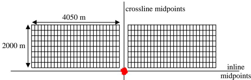
Figure 3. Quad-source midpoint area with OVTs in BP WATS configuration. Width of tiles in inline direction is  $4050/27 = 150$  m; in the crossline direction the width is  $2000/8 = 250$  m.
