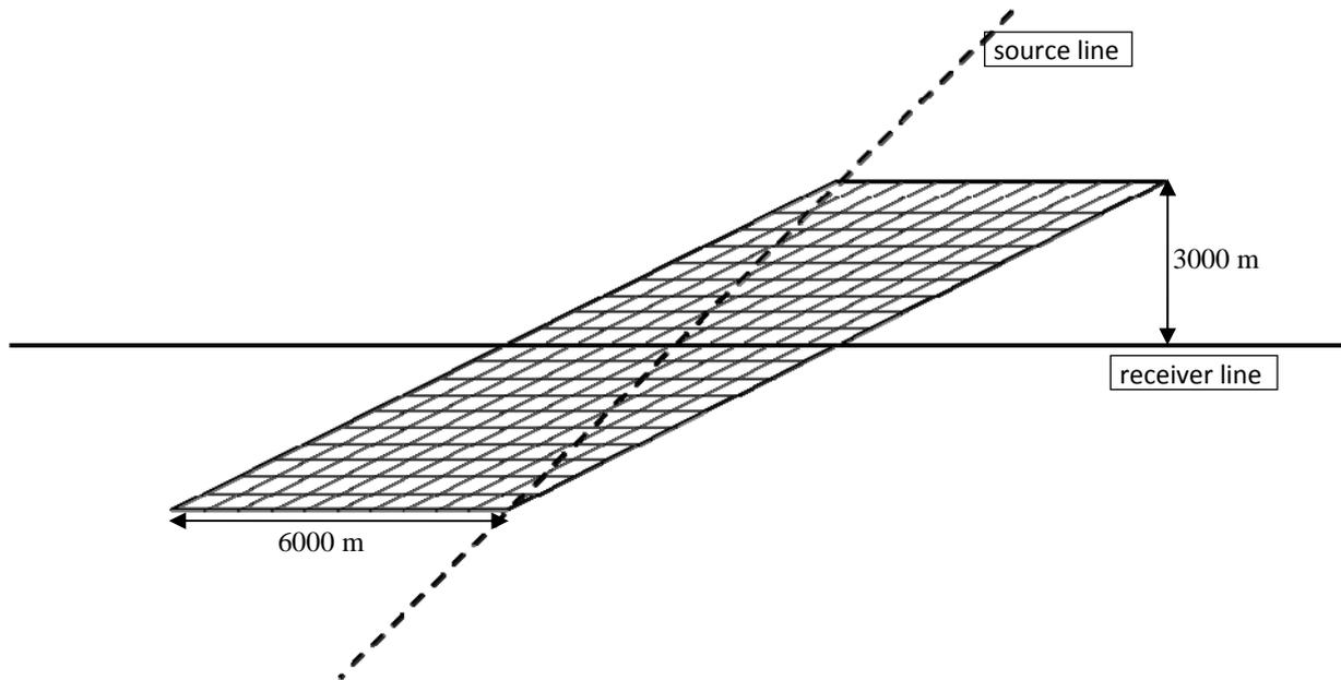
Figure 8. Zig-spread with offset-vector tiles for geometry with active spread length 12000 m, maximum inline and crossline offset 6000 m, receiver line interval 300 m, and source line interval 600 m. There are 10 \* 20 OVTs in this zig-spread, corresponding to a fold of the zig-spreads only of 200. Adding zag-spreads would bring fold to 400.
