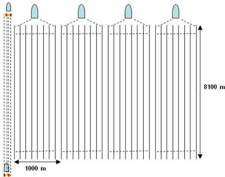
Figure 1. BP WATS configuration with two source vessels with two sources each and a single streamer vessel. The source vessels traverse the same source tracks four times while the streamer vessel moves up over 1000 m each time. Next the whole configuration moves up over 250 m in the crossline direction.
