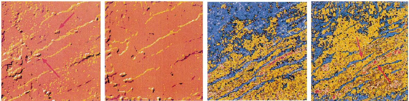
Figure 6. Illumination (left two blocks) and amplitude (right two blocks) produced by brick wall and cross-spread geometries. The cross-spread generates a cleaner image and more sharply defined faults. The brick-wall results are on the left of each pair of displays.
