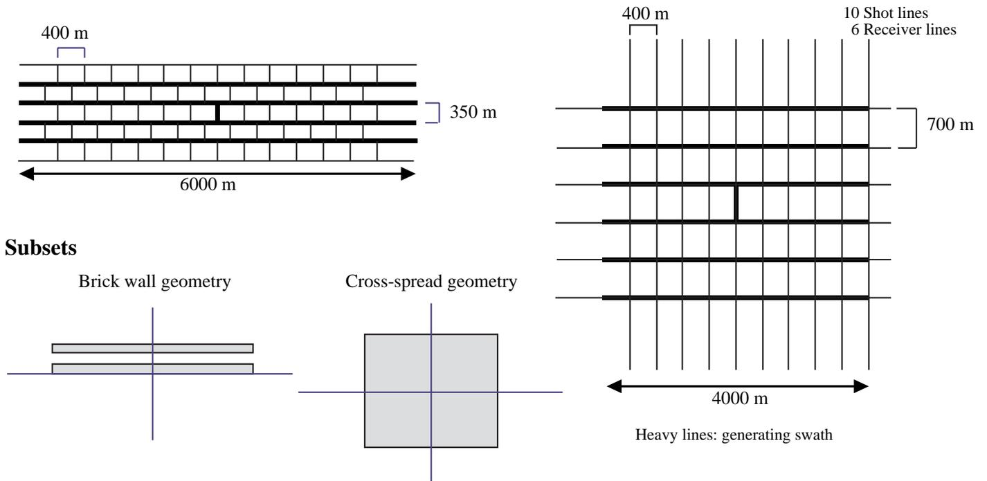
Figure 5. Conventional brick geometry (left) vs. cross-spread geometry (right).
