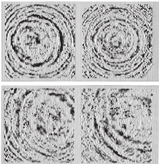
**Figure 2. Time slices through cross-spread illustrate that square cross-spreads maximize spatial continuity: (a) 1700 ms, (b) 2100 ms, (c) 2500 ms, and (d) 2900 ms.**
